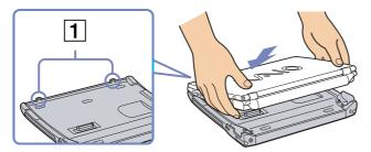
5 Press the bottom of the notebook on the docking station until you hear two clicks. The docking station is now connected to the computer.
